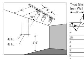
EXAMPLE: With track located 40" from wal and multiple units spaced 38" on center and aimed 60° from horizontal, the illumination on wall 5' 6" from floor will be 48 f.c. beneath units and 47 f.c. between units.
